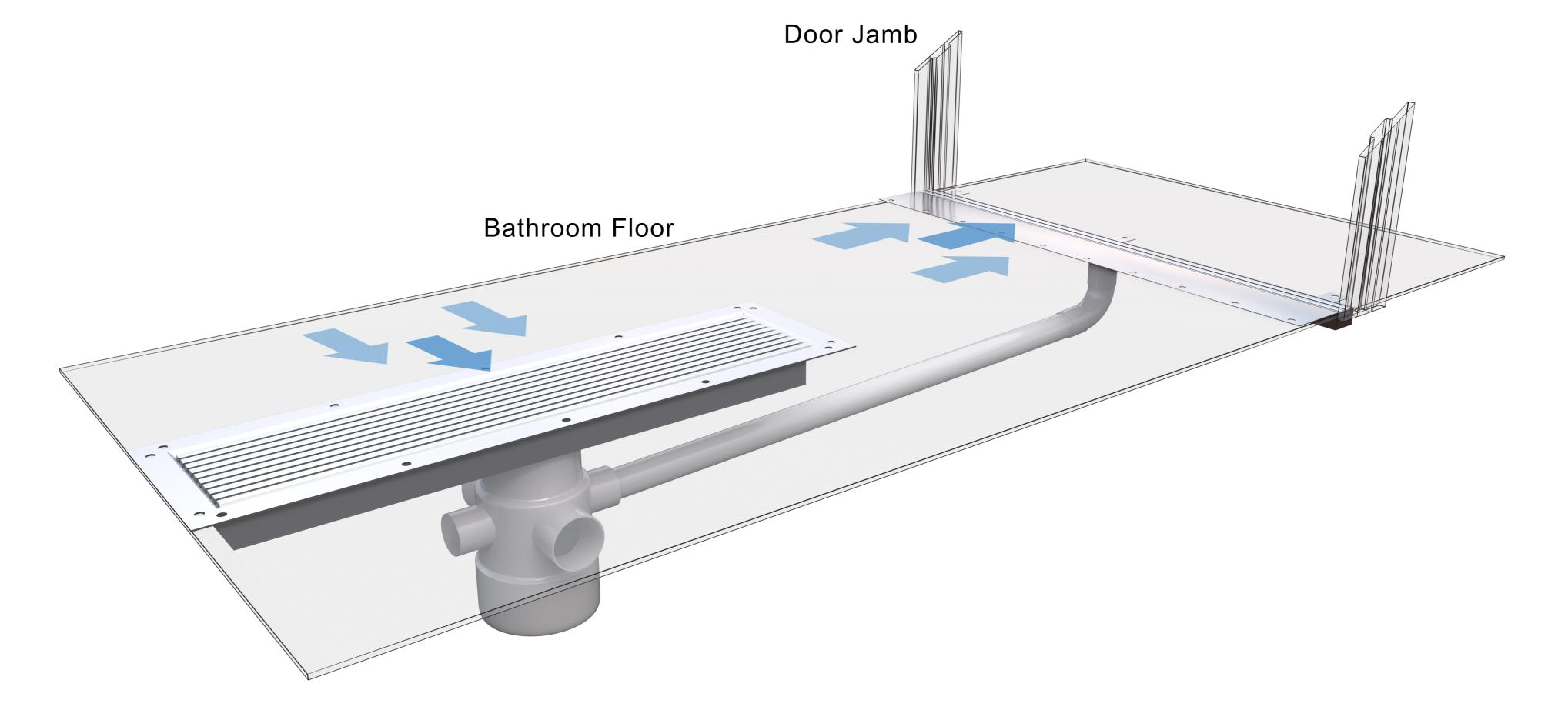
5 - 40mm Emergency Overflow Door Channel Plumbed Into Trapped 4 Way Riser Under Shower Channel
